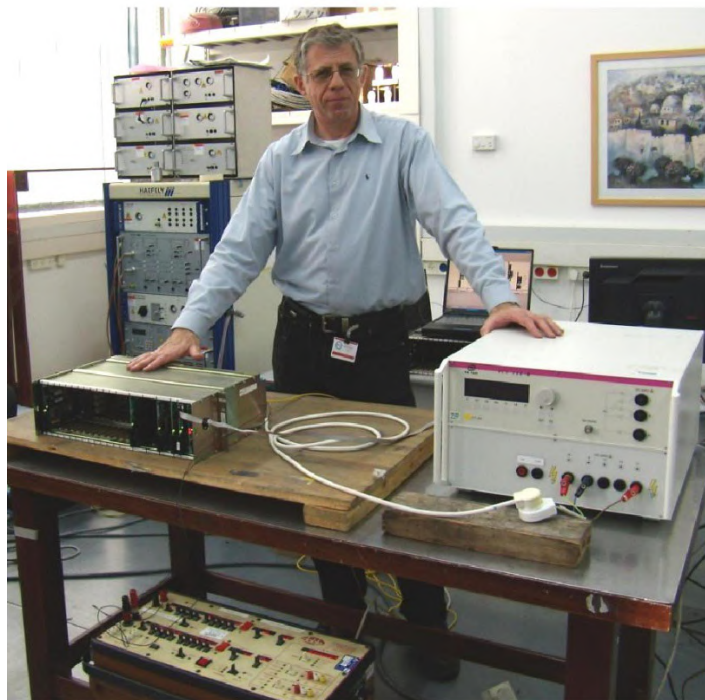
Fig. 10. The author in the process of testing the optical multiplexer (left) type FOCUS (Fiber Optic Communications for Utility Systems) for compliance with IEC standards for electromagnetic compatibility
