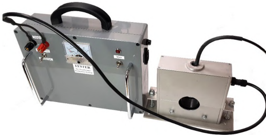
Fig. 19. Simple E3 component simulator for testing serviceability of the system for protection of high-power transformer
