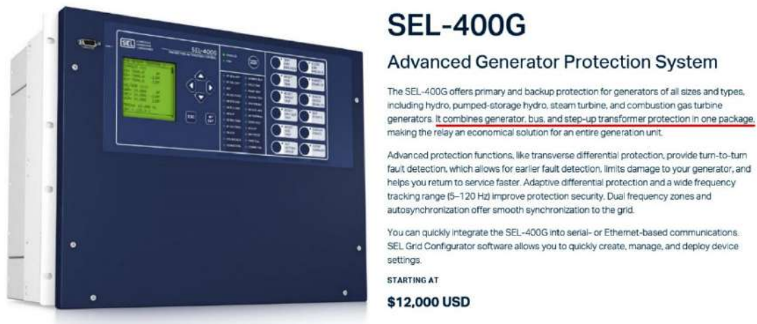
Fig. 1.10. The new SEL-400G digital protection system, concentrated in a single module all protection functions of power station generator; all protection functions of bus bar and all protection functions of step-up power transformer.
