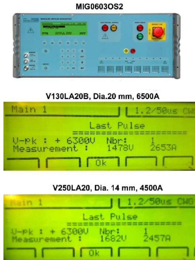
Fig. 4.14. Screenshots of MIG0603OS2 pulse generator when testing varistors V250LA20 (14 mm) and V130LA20B (20 mm) with maximum rated pulse current at 4,500 A and 6,500 A, respectively.
