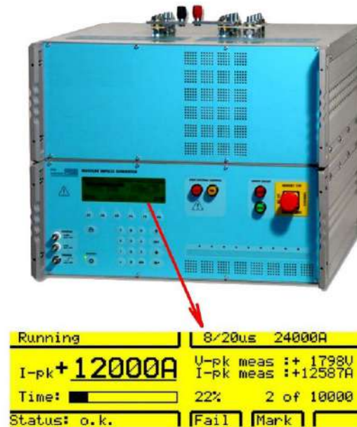
Fig. 4.13. Parameters of test pulse registered by internal measuring circuit of MIG0624 generator (screenshot).
